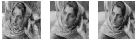
Fig. 5 Performance of Algorithm FISVD for Barbara in different iterations: (a) 1st iteration, (b) 85-th iteration, (c) 172-th (last) iteration.
